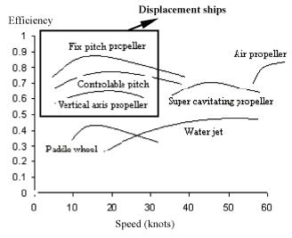
**Figure A2.6** *Efficiency of propulsive devices [31]*
