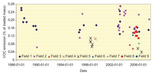
Figure 3.5 VOC emission factor measured during offshore loading in the North Sea
