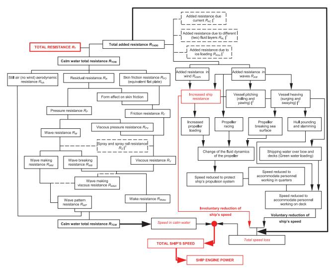
Figure A3.1 The decomposition of total resistance R<sub>T</sub> and effects due to waves and wind loading on displacement type of ships.
