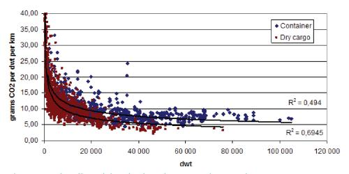
**Figure 6.1** The effect of ship deadweight on CO<sub>2</sub> design index [2]
