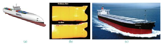
Figure A2.2 (a) Example of a superslender monohull with outriggers (copyright STX Europe, 2008); (b) Axebow design; and (c) 172,000 DWT Capesize bulk carrier Kohyohsan, built with an axe bow for Mitsui O.S.K. Lines, Ltd in 2001.
