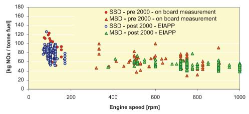
Figure 4.2 NO<sub>x</sub> emission factors from measurement and from EIAPP certificates
