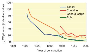
Figure 9.5 Indicative development in maximum ship design transport efficiency
