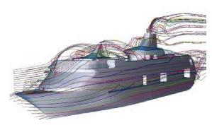
Figure A2.3 A CFD analysis of wind resistance (CFD Norway)
