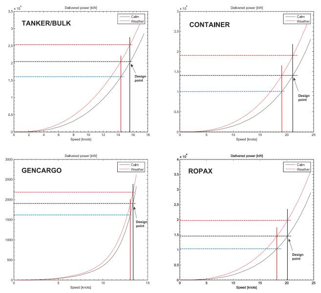
**Figure A3.3** Speed loss (drop) at constant delivered power  $P_D$  or at increased delivered power  $P_D$ , at constant speed, of the advance of vessels in head weather conditions (irregular waves and wind from the same direction 180°) for four different types of ships, according to MARINTEK's 2008 direct model tests database, with the assumption of Beaufort number BN (Bft) = 6 for Tanker/ Bulk, BN(Bft) = 6 for Container, BN(Bft) = 3 for GenCargo, BN(Bft) = 6 for RoPax
